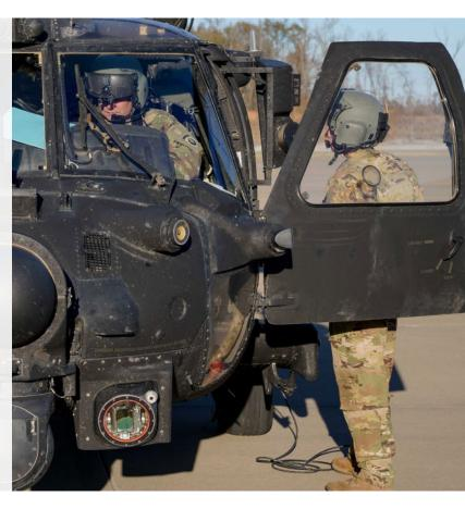
Areté's Lidar for Situational Awareness (LiSA) is a state-of-the-art sensor providing superior pilotage and tactical understanding of hazards, wires, obstacles, flight paths and landing zones in all weather conditions, especially Degraded Visual Environments (DVE). LiSA provides superior range – 2km – and real time 3D spatial awareness of the operational environment and flight guidance at all phases of flight.
